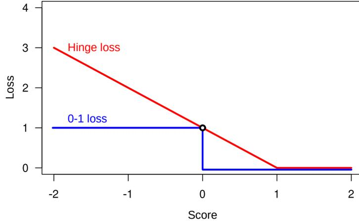
Figure 7: Hinge loss (red) and 0-1 loss (blue) for  $y = +1$ .
